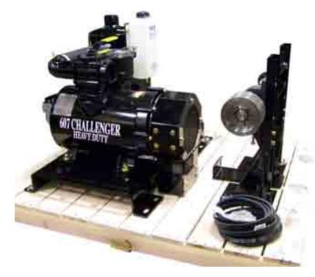
Tighten all bolts, set screws and grease all zerks. Before starting 607 Challenger vacuum pump fill remote oil tank with ISO 68 NVE oil and be sure oil is flowing though lines.
